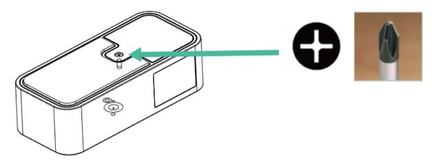
3 Replace the battery with new ones (Li-SiO2 battery, "ER14250", 1/2 AA size x 2 pcs).
